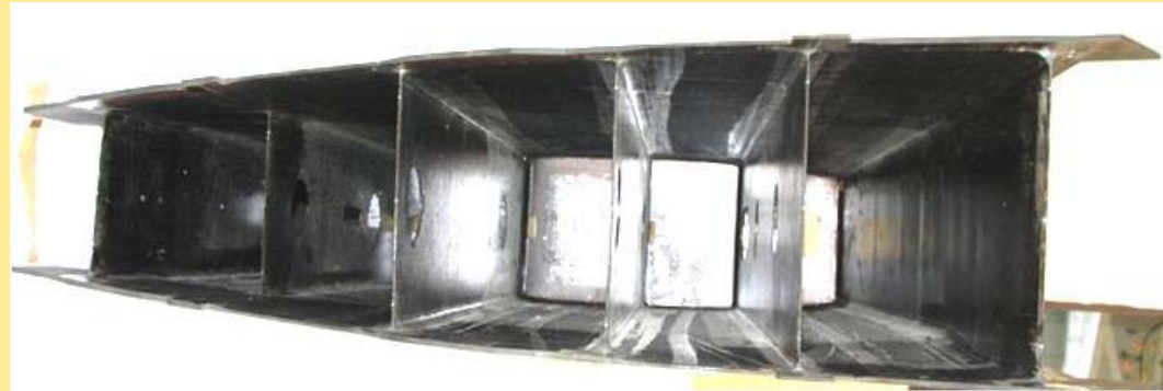
Cocured Inter Spar Box with 6 Spars and a Mid Rib
