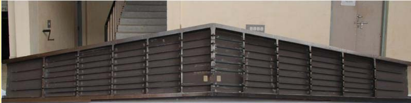
Cocured Inter Spar Box with Bottom Skin With 2 Spars, 11 Ribs, 7 Stringers
