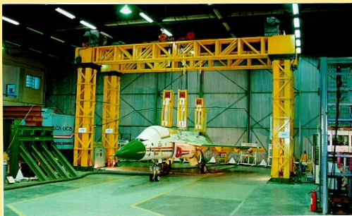
Ground Vibration Test
